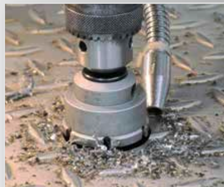
Bohren in Riffelblech
