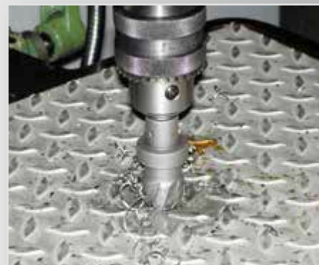
Bohren in Riffelblech
