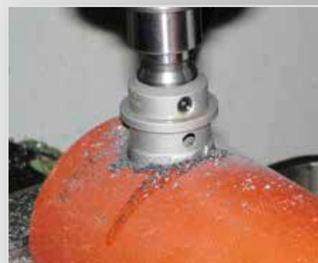
Bohren in Rohre
