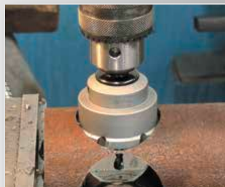
Bohren in Rohre
